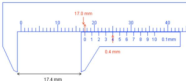
A caliper is a device used to measure distances between two points to high accuracy. The main rule gives you the entire value and the Vernier scale, which slides along the caliper, the next figure
